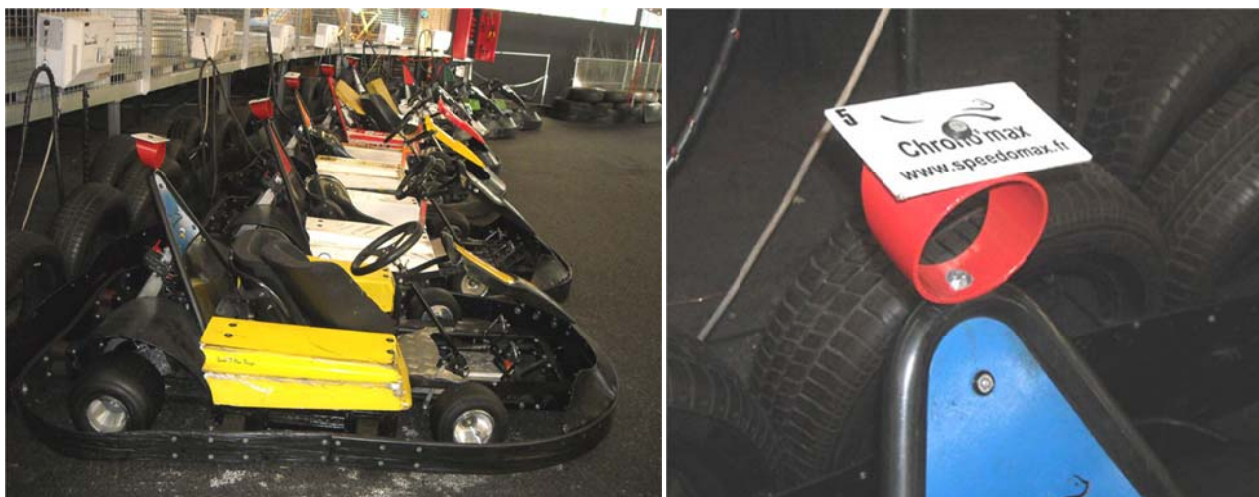
Figure. Example of attaching a kart SPEEDOMAX plate and RFID ChronoMax (Red, PVC pipe of 100 mm!).
