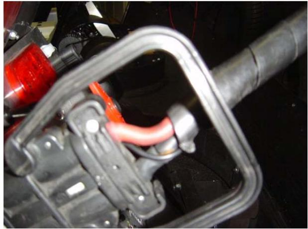
The sockets are asymmetrical and have a flat face. For mounting on the LEFT side of the kart (rear view in the direction of travel), the positive terminal 48 V is found in UP, and the auxiliary contact. The negative-0V is found in BAS.
