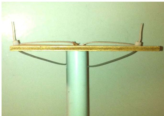
*Figure. Example of attaching a kart: 20mm rigid plastic tube + 2 clamps*
